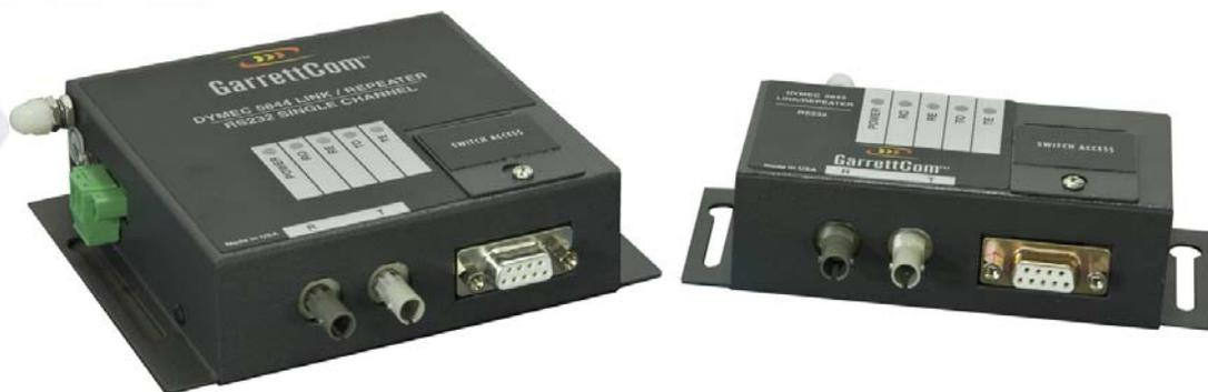
Dymec models 5843 and 5844 are hardened fiber optic Link/Repeaters that convert RS232 or TTL level copper to amplitude based fiber output. Supports data rates from dc to 250k bps, DCE or DTE port configuration and a diagnostic/test mode that allows testing of the copper and fiber connections before the connected IED is active in the network.
